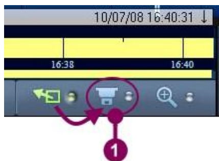
Figure 3-27 The Panning and tilting function of the PTZ camera
