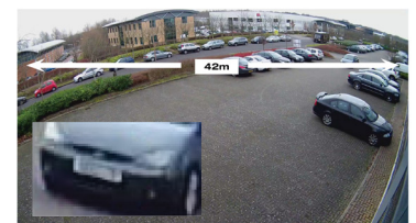
IPR7424ESX3.6 Lens set to 3.3mm Distance to target: 30m
