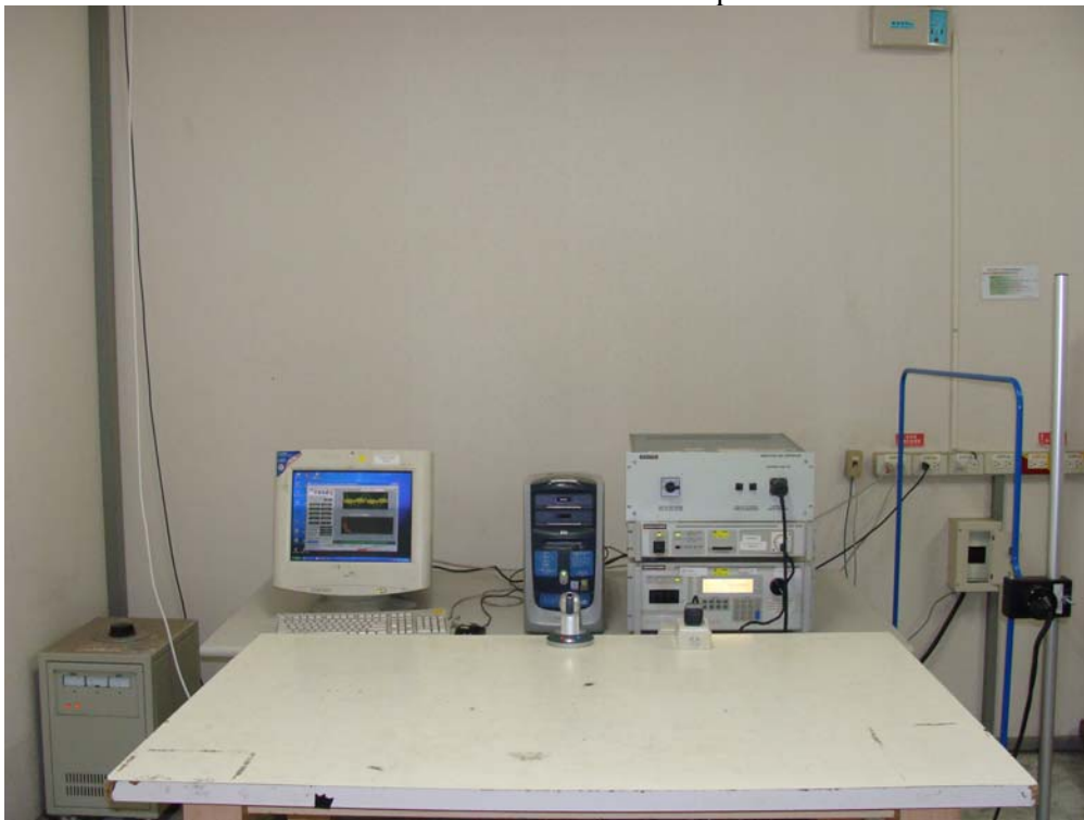
Power Harmonics Test Setup
