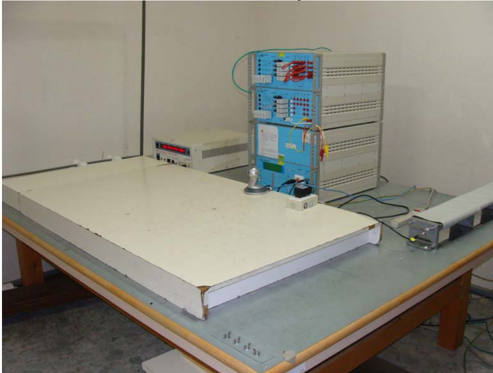
SURGE Test Setup
