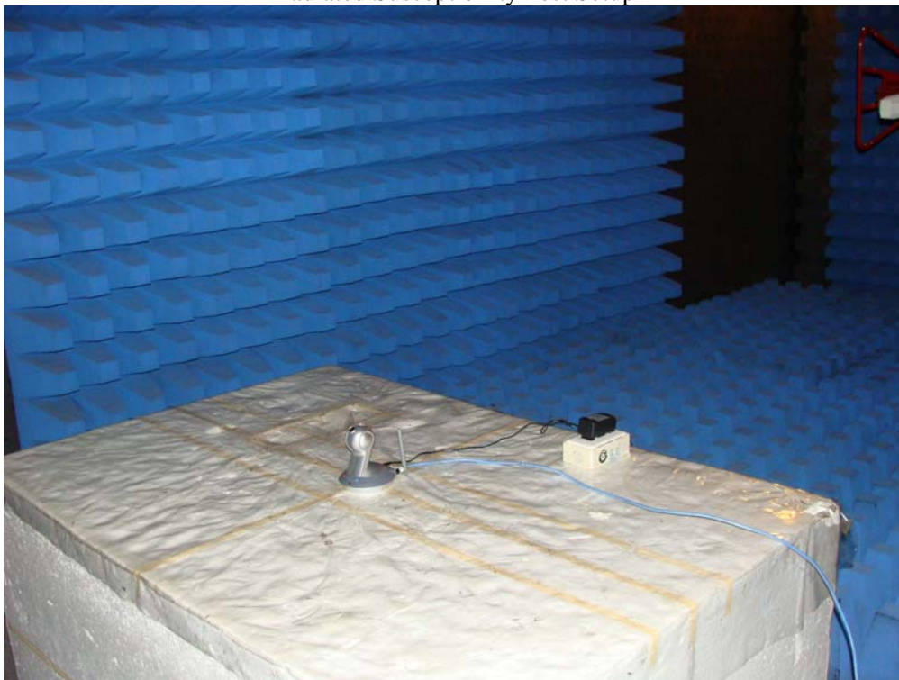
Radiated Susceptibility Test Setup
