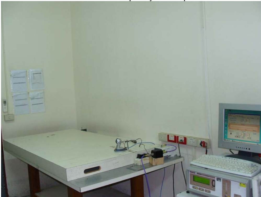
Conducted Susceptibility Test Setup
