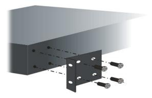
2. After the bracket installation, the VigorSwitch's chassis can be installed in a rack by using four screws for each side of the rack.
